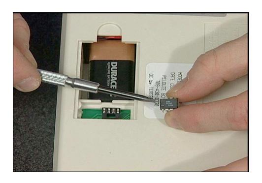
Be careful that the notch is on the correct side of the socket. Check that each pin will slip into the socket.
